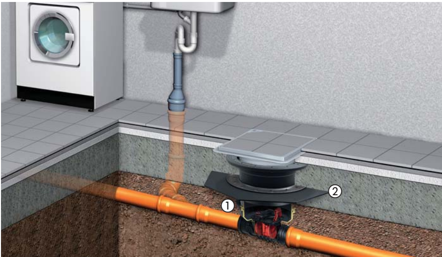
① Backwater valve
